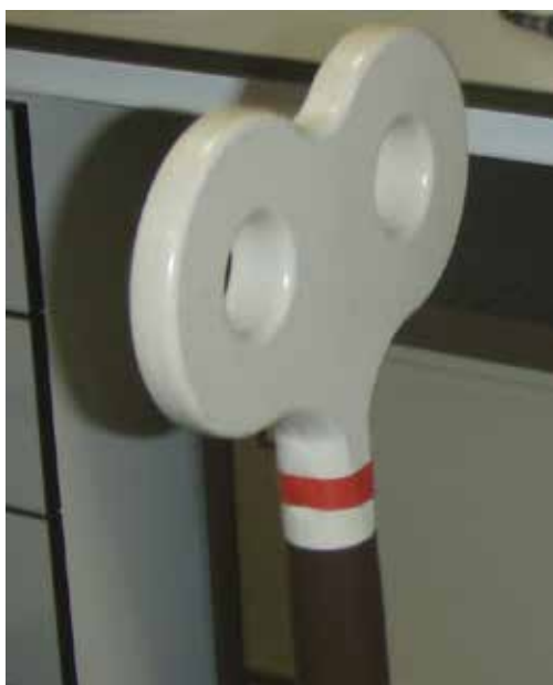
Figure 4.2 — ‘Figure-of-eight’ TMS coil
