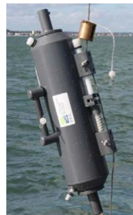
Niskin water bottle attached to winch wire. The brass messenger sits on the wire just above the triggering mechanism. The bottle has been deployed and the caps, top and bottom, are in closed position.
