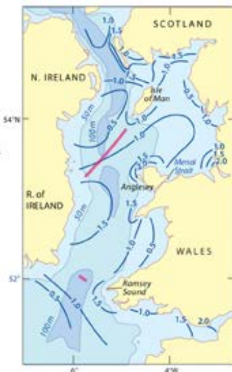
Figure 2 Contours of tidal current speed ( \text{ms}^{-1} ) in the Irish Sea at mean spring tides, superimposed on the bathymetry. The positions of the shelf-sea fronts according to Simpson and Hunter are shown in red. (Current speeds are taken from Bowden (1955))
