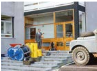
With my equipment for the Menai Strait cable - cable, electrodes and oil drums to buoy the cable during deployment and the lab's Land Rover (EJC 98).
